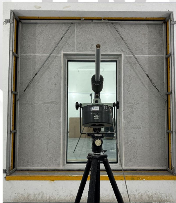
Figure 3 : “S-108 Double Glazed” partition system with 10mm thick tempered glass + 60mm air gap + 12mm thick tempered glass facing the receiving room
