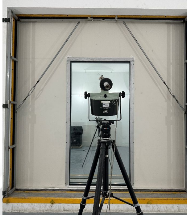
Figure 2 : “S-108 Double Glazed” partition system with 10mm thick tempered glass + 60mm air gap + 12mm thick tempered glass facing the source room
