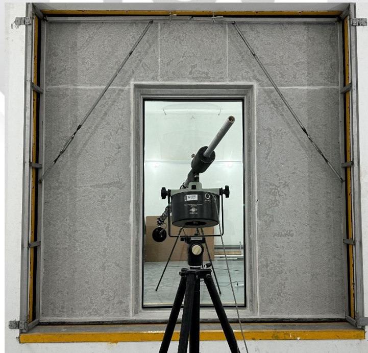
Figure 3 : "S-28 Mini" single glazed partition system with 12mm thick tempered glass facing the the receiving room
