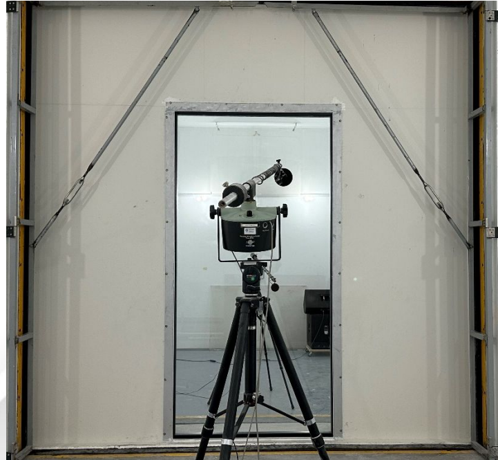
Figure 2 : "S-28 Mini" single glazed partition system with 12mm thick tempered glass facing the source room
