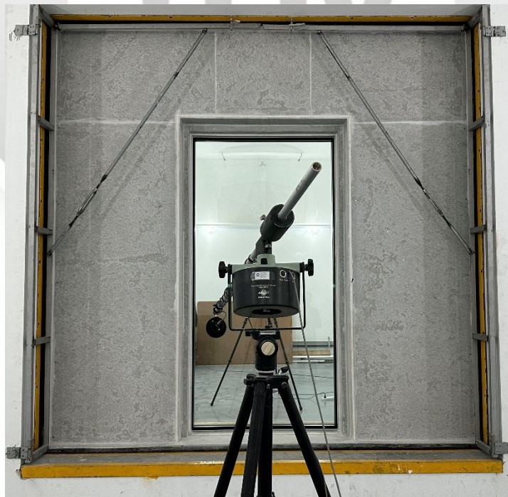
Figure 3 : "S-68 Single Glazed" partition system with 12mm thick tempered glass facing the the receiving room
