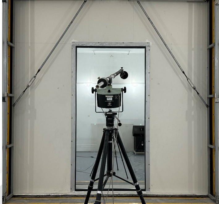
Figure 2 : "S-68 Single Glazed" partition system with 12mm thick tempered glass facing the source room
